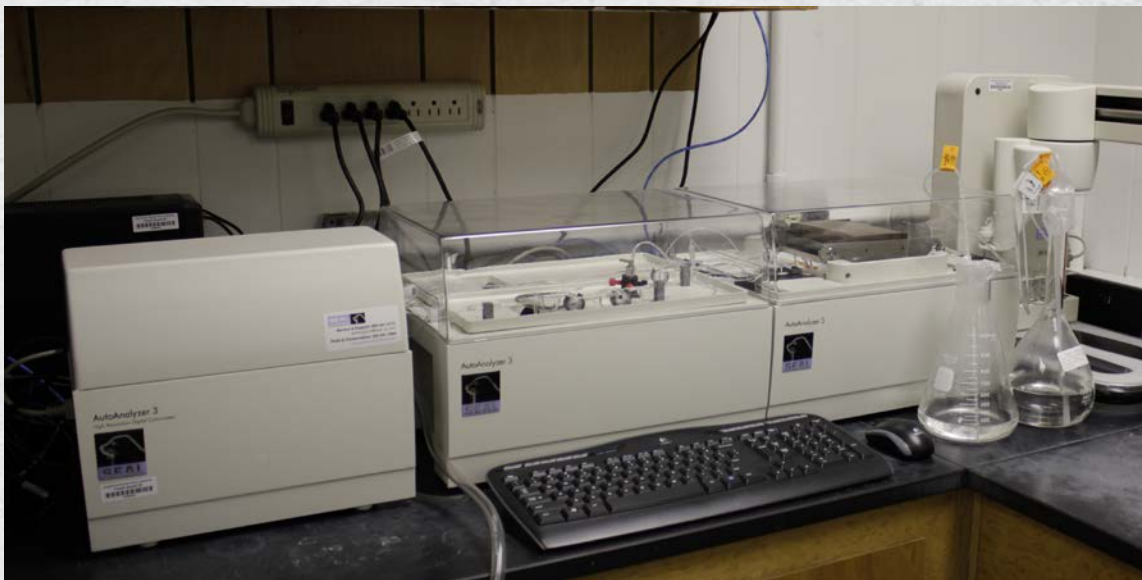
SEAL AutoAnalyzer 3 for nutrient analysis. This equipment has an autosampler for automated analysis, and is capable of detecting analytes at much lower levels than classical wet chemistry techniques.
